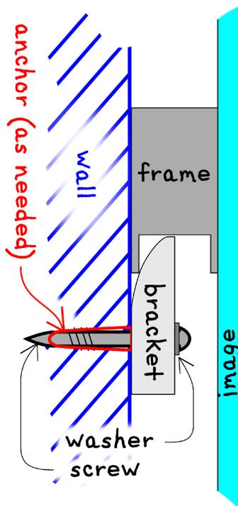
3. While holding the bracket with the bottom edge on the line and the curved edge up and toward the wall (as in Figure 2), place one screw in the hole and tap to mark the wall for the drill.
